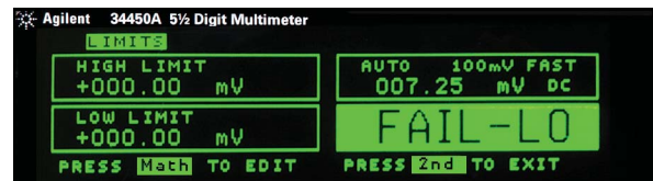
Four-quadrant limit test display
